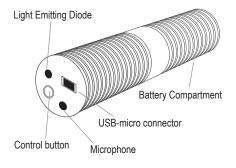
Figure 1: Edic-mini Tiny Model B26
